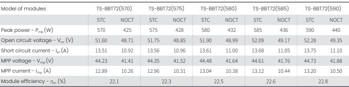
STC (Standard Testing Conditions): Irradiance 1000W/m<sup>2</sup>, Cell Temperature 25 °C , Spectra at AM1.5
